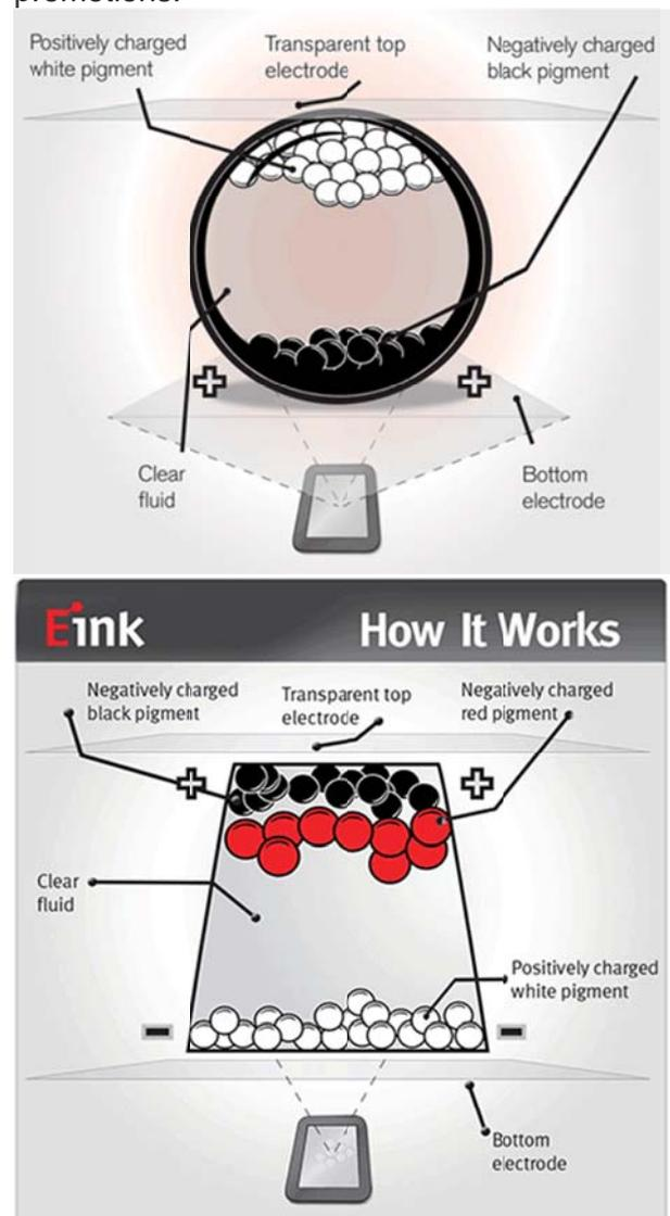
Spectra is made up of millions of tiny microcups, about the thickness of a human hair. Each microcup contains positively charged white particles and negatively charged black and red particles suspended in a clear fluid.
